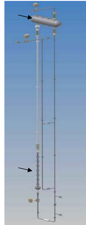
Figure 1.1 An illustration of the GENESIS facility where the top and bottom arrows indicate the steam separation vessel and reactor core respectively
