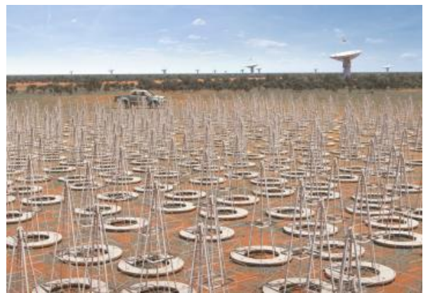
Antennas of the Square Kilometre Array (SKA) which will become the largest and most sensitive radio telescope. The design is based on the Dutch LOFAR telescope
