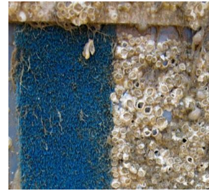
Figure 2 – Comparison of surface protected and unprotected by Micanti antifouling
