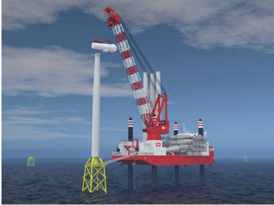
Figure 1: Wind turbine installation vessel
