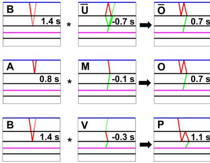
Figure 9: Illustrations of the events in the upgoing focusing function and Green's function after step 3. Events  $\bar{O}$  and  $P$  are found in the second term, while event  $O$  is a contribution of the third term.
