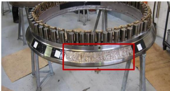
**Fig 1:** Spallings at the inner ring in regions of highest contact pressure.
