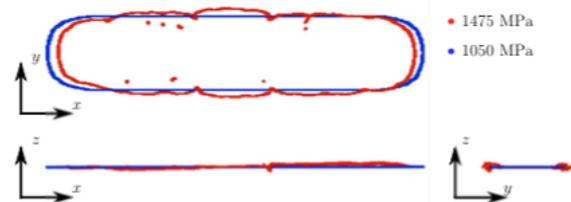
*Example of two expanding dislocation shear loops under different applied shear stress levels  $\sigma_{xz}$ , starting from different initial sizes.*
