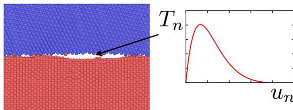
*Interface decohesion at iron/precipitate interface and shape of cohesive law relating tractions  $T_n$  to separations  $u_n$  at interface.*
