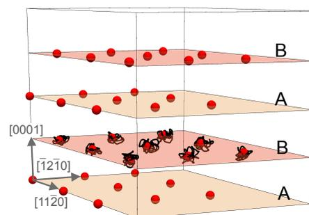
Sketch of ab initio MD trajectories in a hcp cell (with ABAB... stacking). Such calculations have been employed in [Zhang et al., PRB 2018] to compute highly-accurate finite-temperature SFEs from ab initio.
